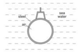
What causes the upthrust on the submarine?
