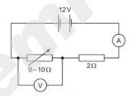
The resistance of the variable resistor is changed from zero to its maximum value.
