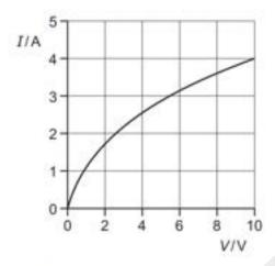
Since the graph is not a straight line, the resistance of the lamp varies with V.
