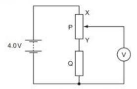
The slider on the potentiometer is moved from X to Y and a graph of voltmeter reading V is plotted against slider position.
