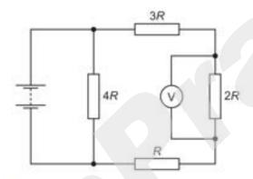
The voltmeter reading is 2 V.
