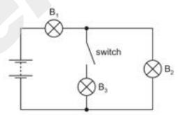
Initially the switch is closed. The switch is then opened and lamp B3 goes out.
