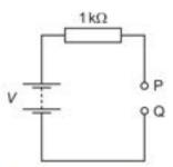
A student attempts to measure the potential difference (p.d.) between points P and Q using two voltmeters, one at a time. The first voltmeter has a resistance of  $1\,\mathrm{k}\Omega$  and the second voltmeter has a resistance of  $1\,\mathrm{M}\Omega$ .
