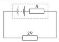
What is the ratio power in external resistor power in internal resistance?
