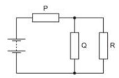
The battery, of negligible internal resistance, supplies a total power of 12W.
