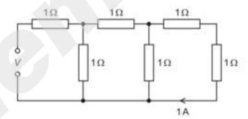
The current passing through the end resistor is 1 A.
