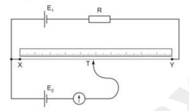
The contact T is placed on the wire and moved along the wire until the galvanometer reading is zero. The length XT is then noted.
