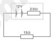
What is the power dissipated in the  $13\Omega$  resistor?
