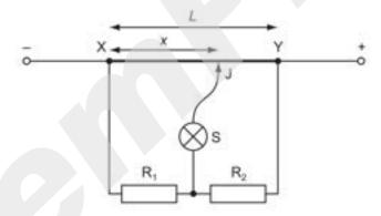
To determine the ratio  $\frac{V_1}{V_2}$  of the potential differences across R<sub>1</sub> and R<sub>2</sub>, a point is found on XY at which the lamp is off. This point is at a distance x from X.
