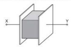
The cube has volume V and is made of a material with resistivity  $\rho$ . The connections to the cube have negligible resistance.
