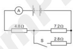
When S is open, the reading on the ammeter is 250 mA.
