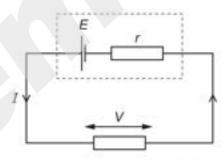
The current in the circuit is I and the potential difference (p.d.) across the external resistor is V.
