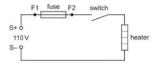
Owing to a fault in the system, power is not supplied to the heater. A technician diagnoses the fault using a voltmeter.
