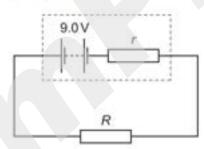
A charge of 6.0 C flows through the resistor in a time of 2.0 minutes causing it to dissipate 48 J of thermal energy.
